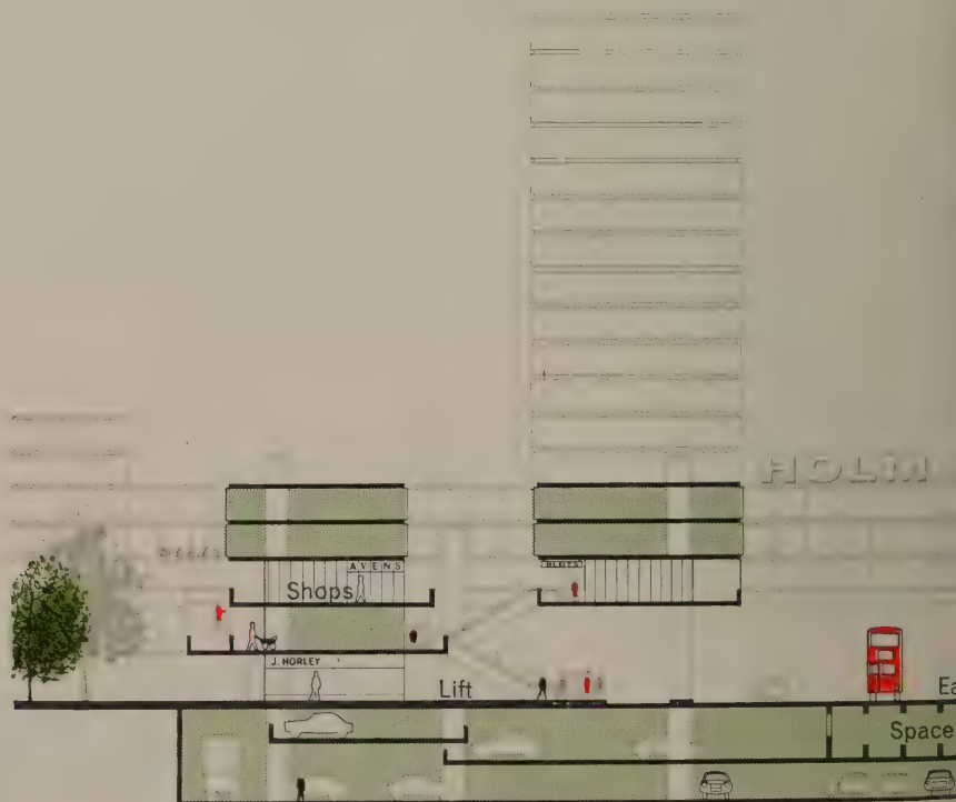
184 The design for complete redevelopment. Sectional view (BB on Figure 182) showing the east-west two-way road with escalators down to the bus lay-bys, and the ground level open space with housing blocks in elevation behind.
